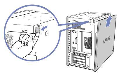
Always wait for the internal parts of the system unit to cool down before removing the side panel.
